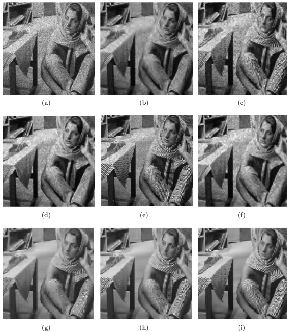
Fig. 3: Synthetic Barbara images obtained for various despeckling methods, (a) Noisy image ( NV = 0.1 ), (b) Contourlet, (c) SWT_Cauchy, (d) SWT_GFD, (e) DWT-Cauchy, (f) Hybrid, (g) Thresholding, (h) Modelling, (i) Proposed.
